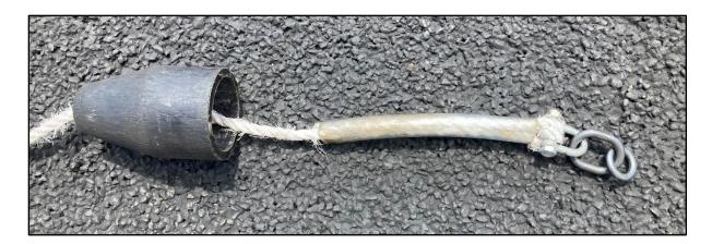
It is important that the plastic tube is pushed up to the D-shackle when attaching the rings to the release. The black protector sleeve should be pushed up towards the end of the rope noting that it is a loose fit and will slide back under its own weight when on the ground. Once airborne the airflow moves the sleeve towards the end of the rope and after release the sleeve slides all the way to the end and protects the rings.
