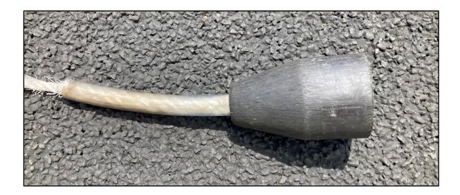
The protector sleeve slides to the glider end of the rope after release, where it adequately conceals and protects the rings from abrasion.
